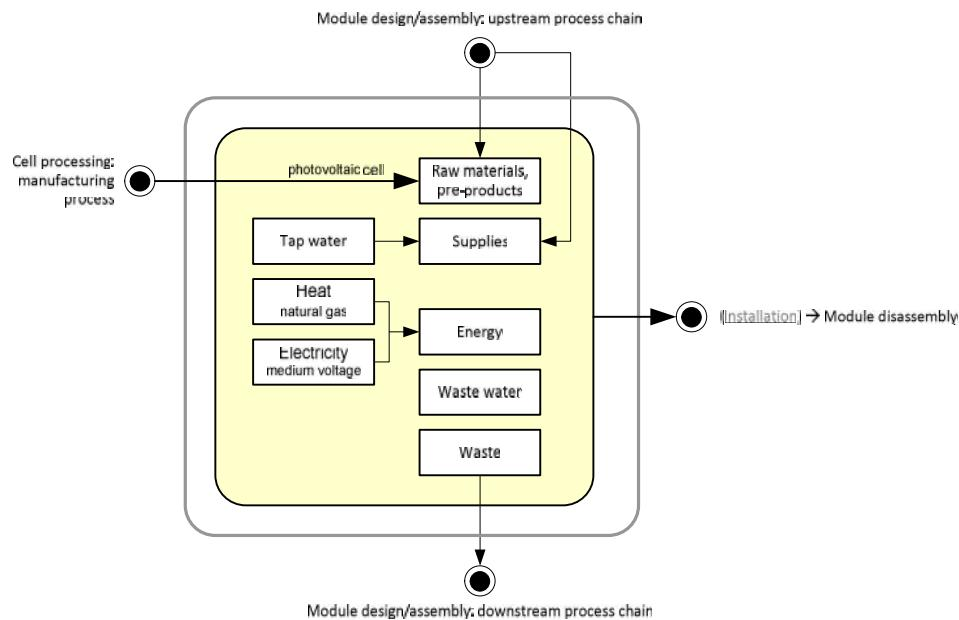
Figure 3.17: sc-Si and mc-Si photovoltaic module production: balance model of manufacturing process
