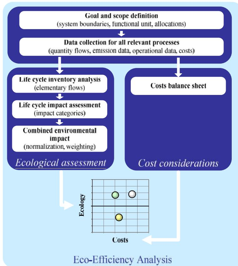
Figure 2.1: Steps for considering the joint environmental and economic impact within the context of the eco-efficiency analysis
