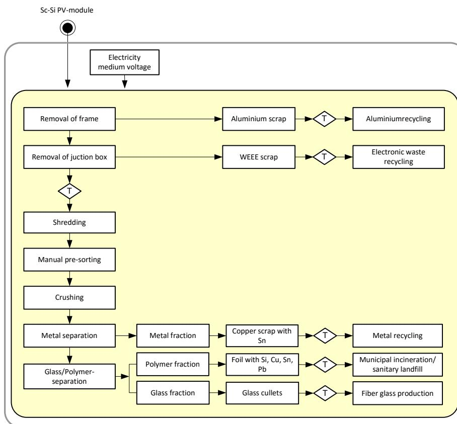
Figure 3.23: sc-Si and mc-Si photovoltaic module production: balance model of module disassembly process
