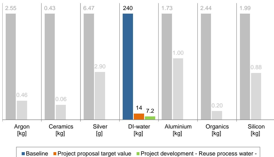
Figure 6.9: Reuse process water: reduction of waste and resource consumption for one sc-Si PV-module (60 6-inch solar cells)
