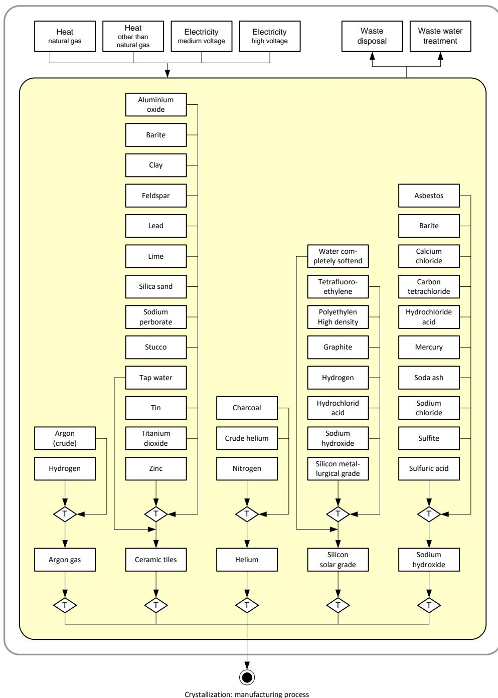
Figure 3.3: Multi-crystalline silicon (mc-Si) production: balance model of upstream process chain
