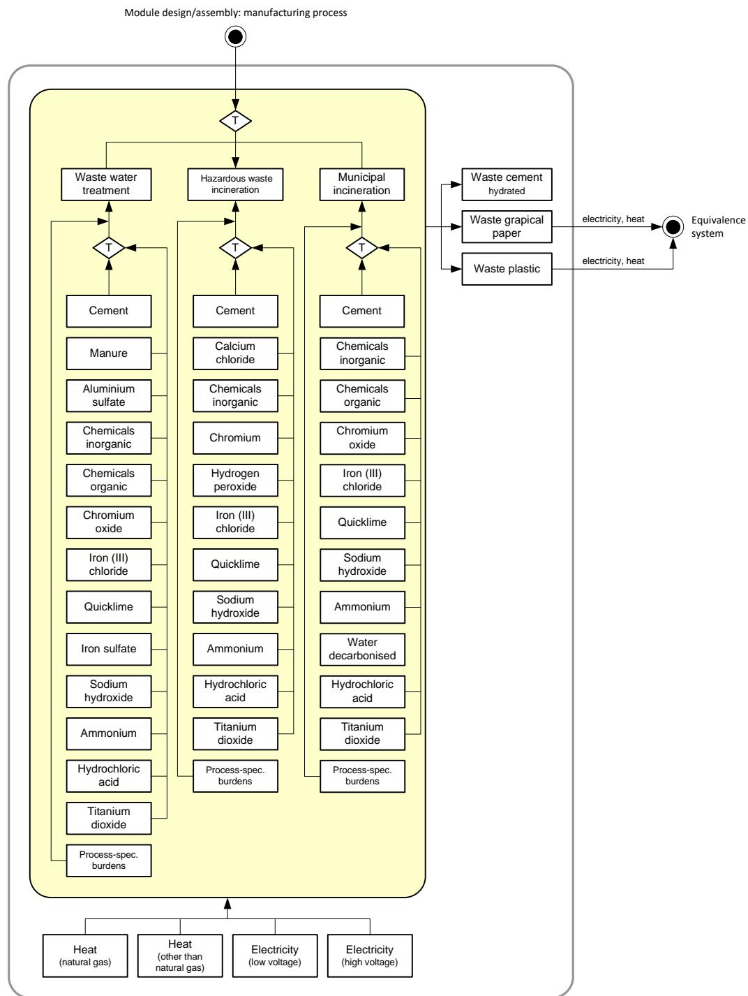
Figure 3.22: NICE module Gen. 2 production: balance model of downstream process chain
