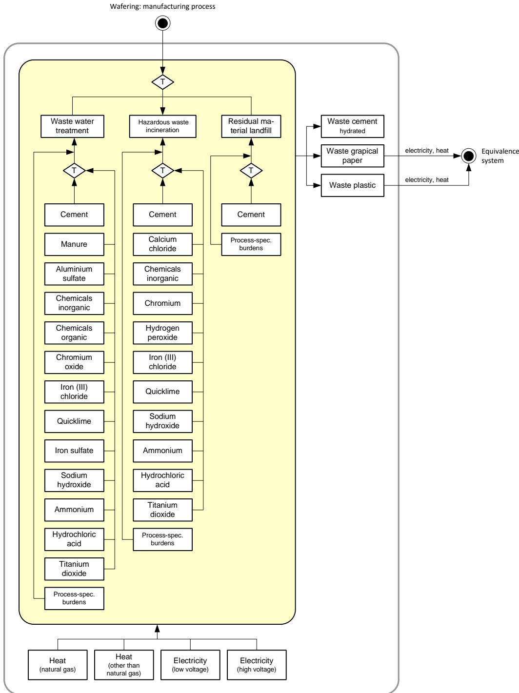
Figure 3.14: sc-Si and mc-Si photovoltaic cell production: balance model of downstream process chain
