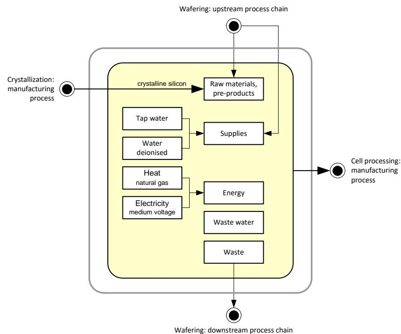
Figure 3.8: sc-Si and mc-Si wafer production: balance model of manufacturing process
