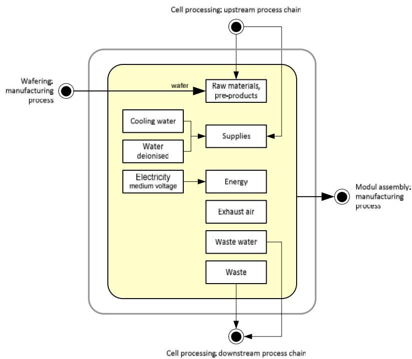
Figure 3.12: si-Si photovoltaic cell production: balance model of manufacturing process
