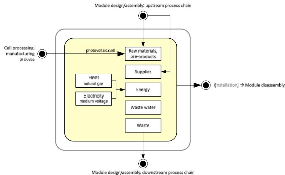
Figure 3.21: NICE module Gen. 2 production: balance model of manufacturing process
