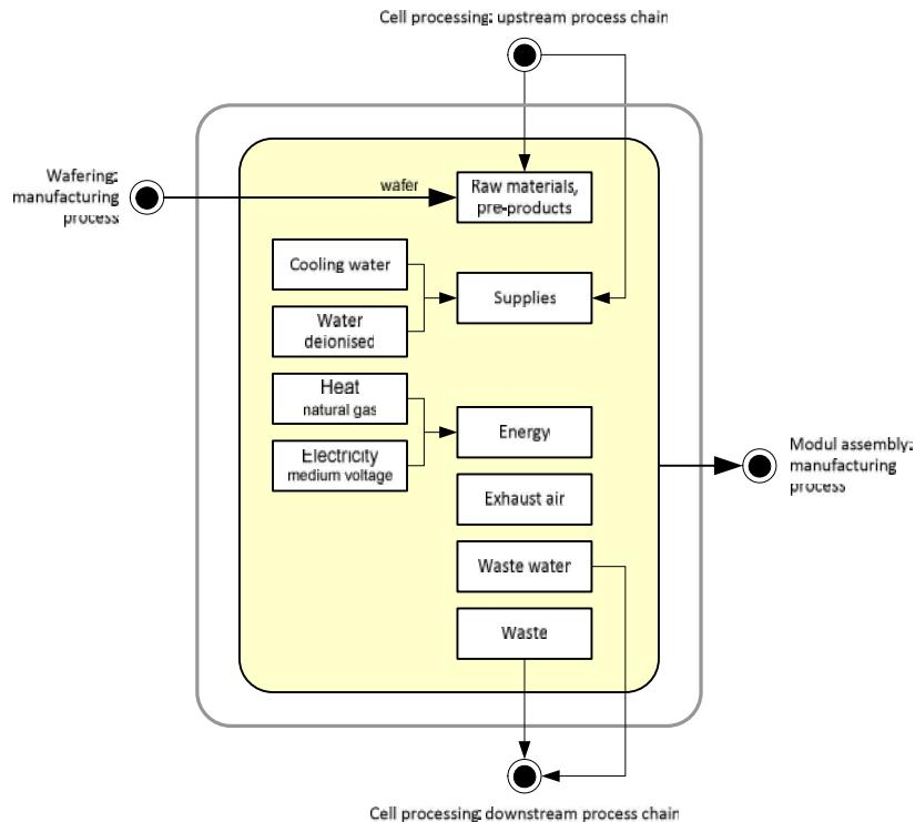
Figure 3.13: mc-Si photovoltaic cell production: balance model of manufacturing process
