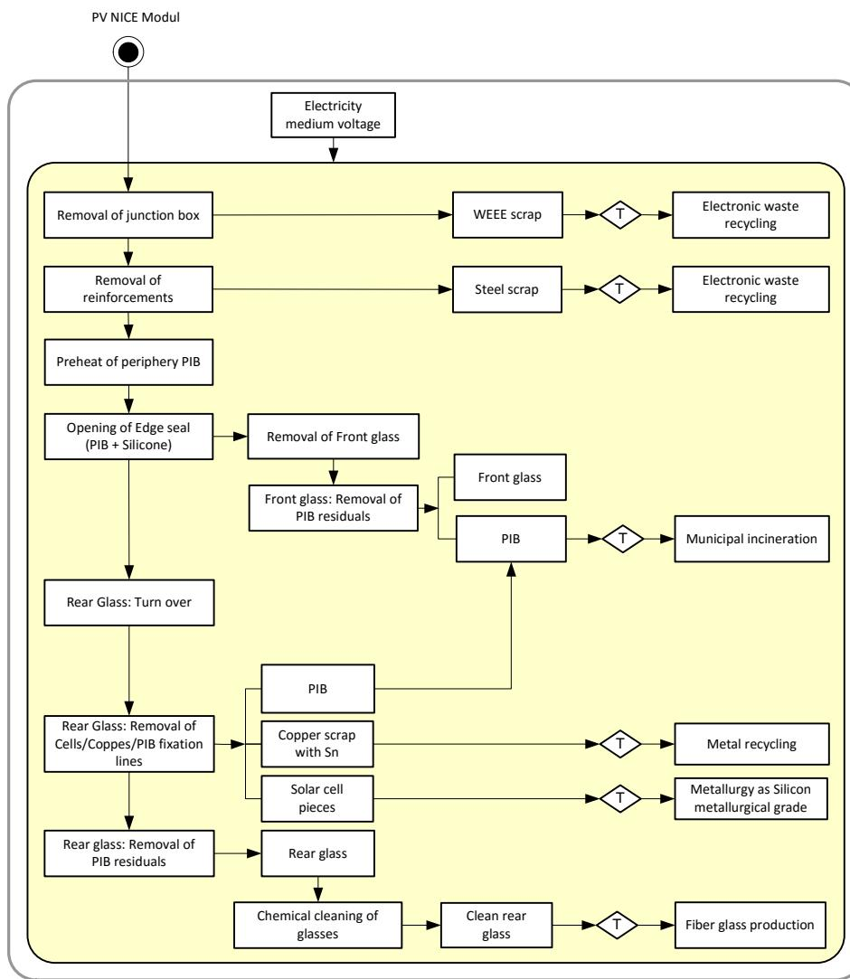
Figure 3.24: NICE PV-module production: balance model of enhanced module disassembly process
