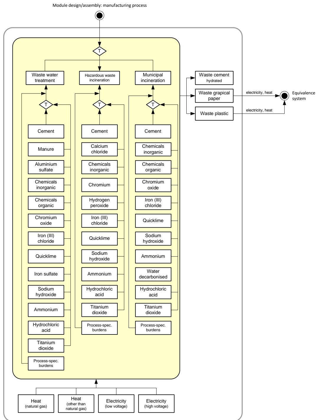
Figure 3.18: sc-Si and mc-Si photovoltaic module production: balance model of downstream process chain
