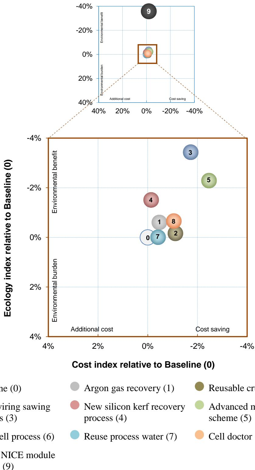
Figure 9.2: Eco-efficiency portfolio for sc-Si PV modules
