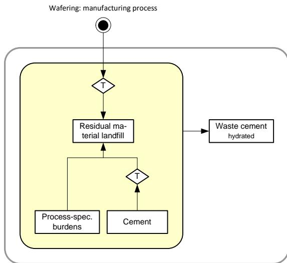
Figure 3.9: sc-Si and mc-Si wafer production: balance model of downstream process chain
