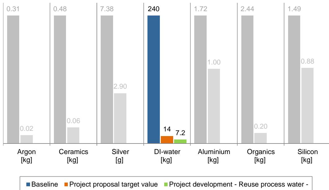
Figure 6.10: Reuse process water: reduction of waste and resource consumption for one mc-Si PV-module (60 6-inch solar cells)
