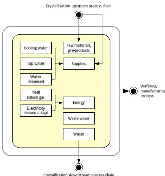
Figure 3.4: Single-crystalline silicon production: balance model of manufacturing process
