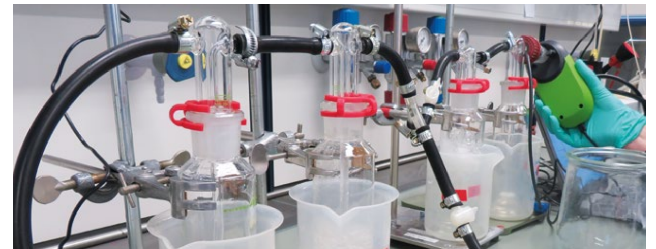
Measuring the test bacteria solution with the airco well® sensor
