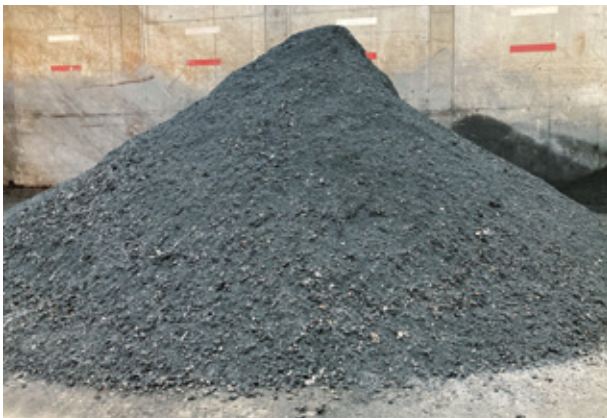
Residual mineral fraction of the bottom ash after ash treatment
