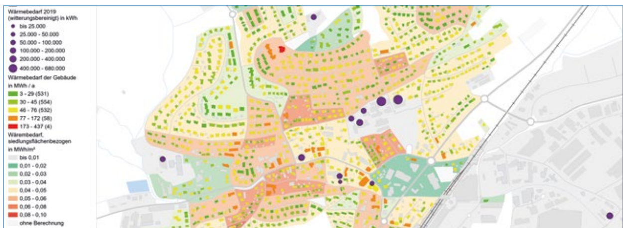
Heat register – heat demand of buildings in the town centre of Erbach
